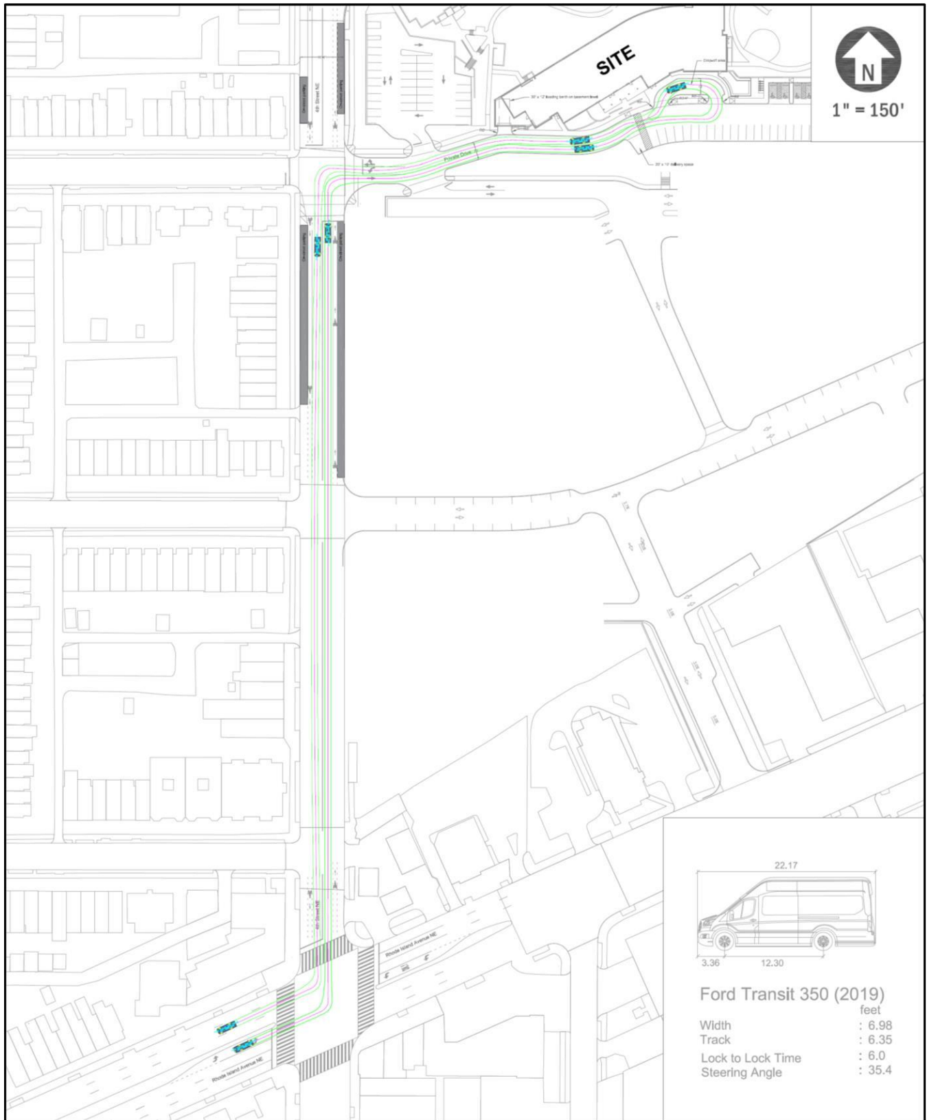
Figure 14: 22' Transit Van Inbound and Outbound Turning Maneuvers between Rhode Island Avenue and Drop-off Area
