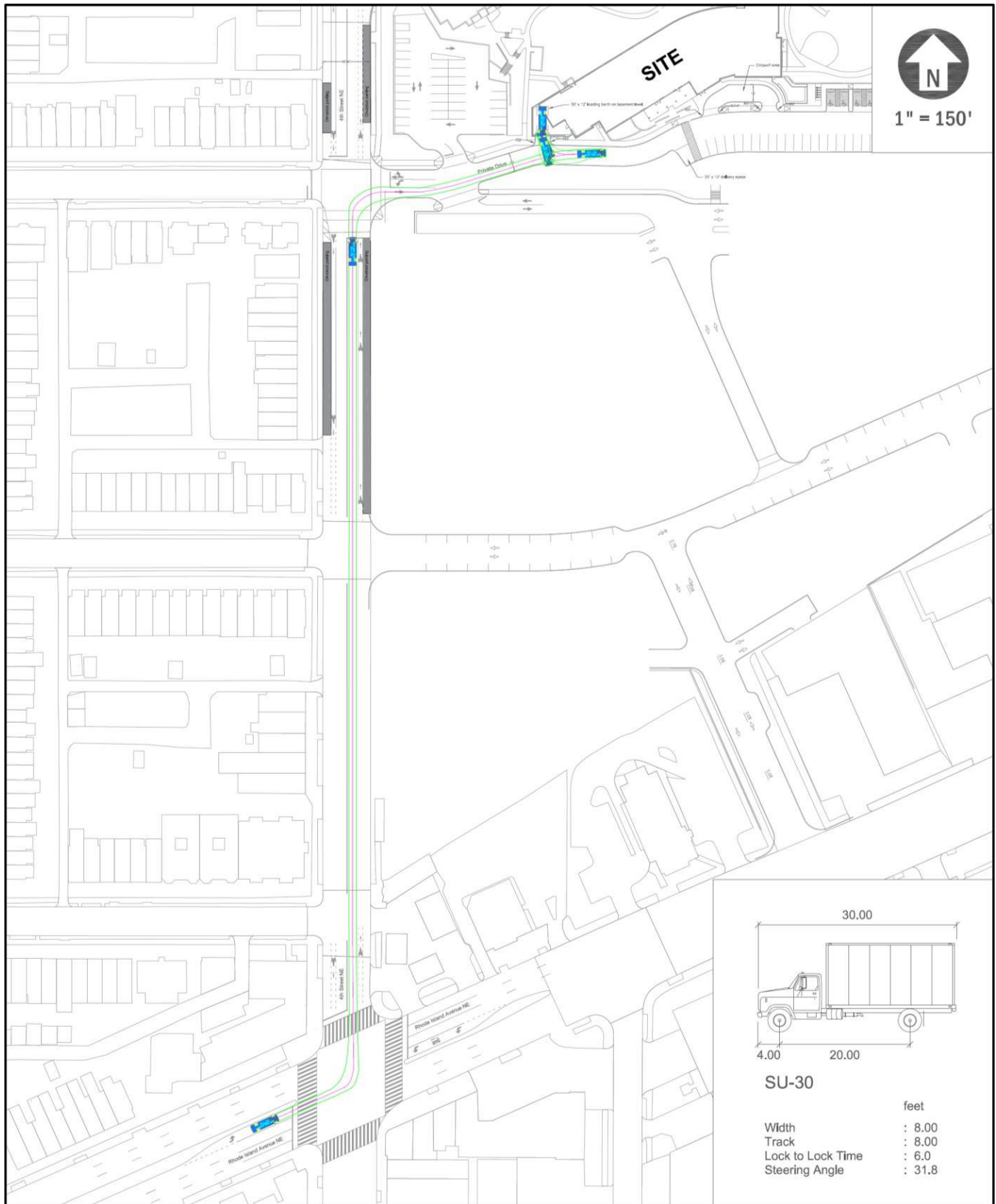
Figure 11: SU-30 Inbound Turning Maneuver from Rhode Island Avenue to Loading Berth
